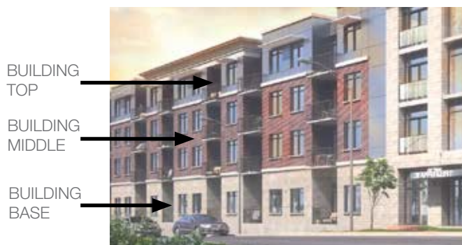
Figure 12: Tall buildings should be designed with stepped down built form that includes a base, middle and upper profiles to avoid overbearing massing
